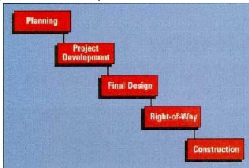
Fig.3.1 Process of Highway Planning
